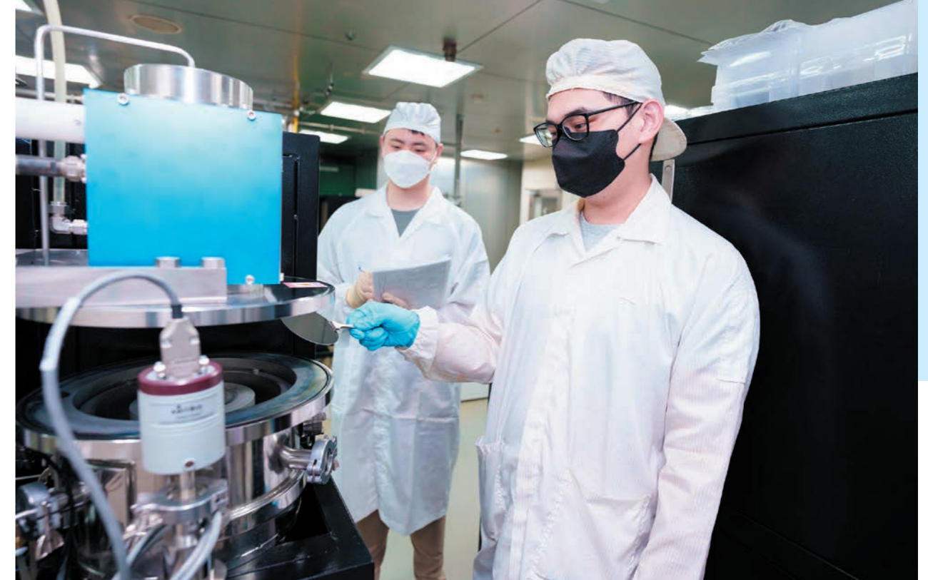
..... A silicon wafer with a 5 nm-thick dielectric layer is going to locate in the chamber of Inductively Coupled Plasma Reactive-Ion Etching (ICP-RIE) system for drying etching process
